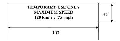
Upper case letters shall be at least 5 mm high and the numbers "120" and "75" shall be at least 20 mm high with the elements that make up each character of the number at least 3 mm line thickness. Lower case text shall at least have a line height of 5 mm. All text shall be enclosed in a border and be on a background of contrasting colour.
