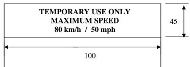
Upper case letters shall be at least 5 mm high and the numbers "80" and "50" shall be at least 20 mm high with the elements that make up each character of the number at least 3 mm line thickness. Lower case text shall at least have a line height of 5 mm. All text shall be enclosed in a border and be on a background of contrasting colour.
