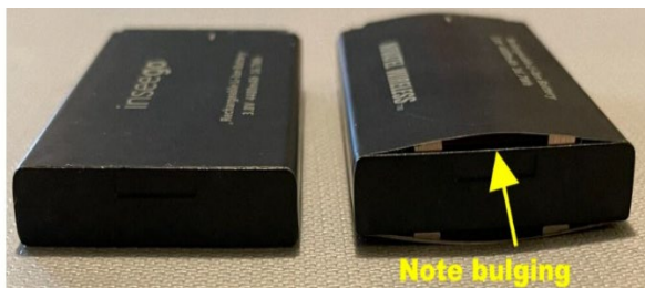
Figure 1 Battery with bulging resulting in internal cells exposed meets definition of rupture.
