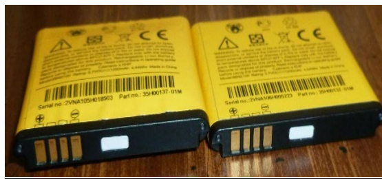
Figure 2 Battery with bulging (no cells exposed) would not meet definition of rupture
