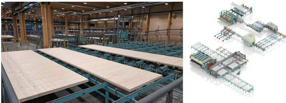
Figure 7: Technological line in the company Stilles, for the production of cross laminated timber panels
