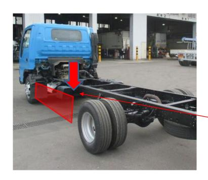
A truck running without a load-carrying platform is dangerous to other road users, because it doesn't have Protector between LPD and chassis frame, which would otherwise prevent them, if collided, from diving under the platform.
