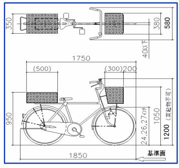
To prevent the cycle structure from diving under the lower part of the LPD when the cyclist fell over, it is appropriate to set LPD's ground clearance to 450mm or less.
