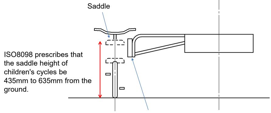
This makes that the effectively designed structure of LPDs is the one that pushes the child away with a flat plane between the height of 450 and 650mm from the ground.
