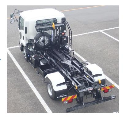
The upper edge of LPD shall not be more than 350 mm below that part of the structure of the demountable body.
