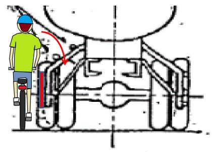
If the cyclist collides with the LPD in the lower part of the body, they might fly over the LPD to tumble beneath the chassis.
