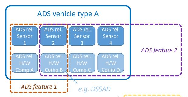
The ADS vehicle type is specified by a dedicated ADS architecture defined by an ADS relevant hardware/ sensor layout, which is outlined in the approval of the ADS vehicle type.
