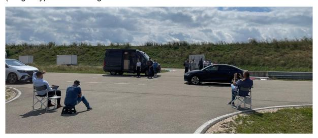
Scenario 2 ("use case 4"): Zebra-crossing, EV passing by with 33 km/h Same scenario as the first but with slightly over 30 km/h
