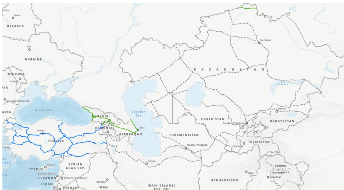
Map 5 Minimum useful siding length meter (dotted grey: no parameters data received, blue: data received but under analysis, green: 750 m minimum)
