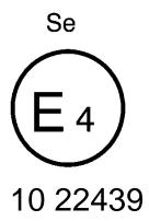
The belt bearing the above approval mark is a special type belt ("S"), fitted with an energy absorber ("e") and approved in the Netherlands (E 4) under the number 1022439, this Regulation already incorporating the 10 series of amendments at the time of approval.
