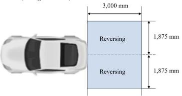
6.28.5.2. The patterns of the reversing projections shall start with their closest edge within a rectangle, symmetrical to the median longitudinal plane and adjacent to the extreme outer edge of the vehicle a width of 1,000 mm and a length of 3,750 mm (see figure below).
