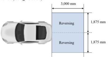
6.27.5.2. The patterns of the reversing projections shall start with their closest edge within a rectangle, symmetrical to the median longitudinal plane and adjacent to the extreme outer edge of the vehicle, having a length of 1,000 mm and a width of 3,750 mm (see figure below).
