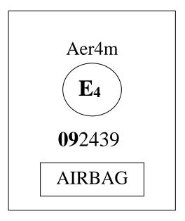
The ... 06, 07, 08 or 09 series of amendments at the time of the approval. This safety-belt has to be fitted to a vehicle equipped with an airbag in the given seating position."
