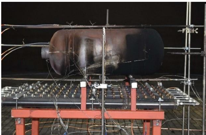
Figure 18 Pre-Test Cylinder Mounted Above the Burner for Thermal Mapping
