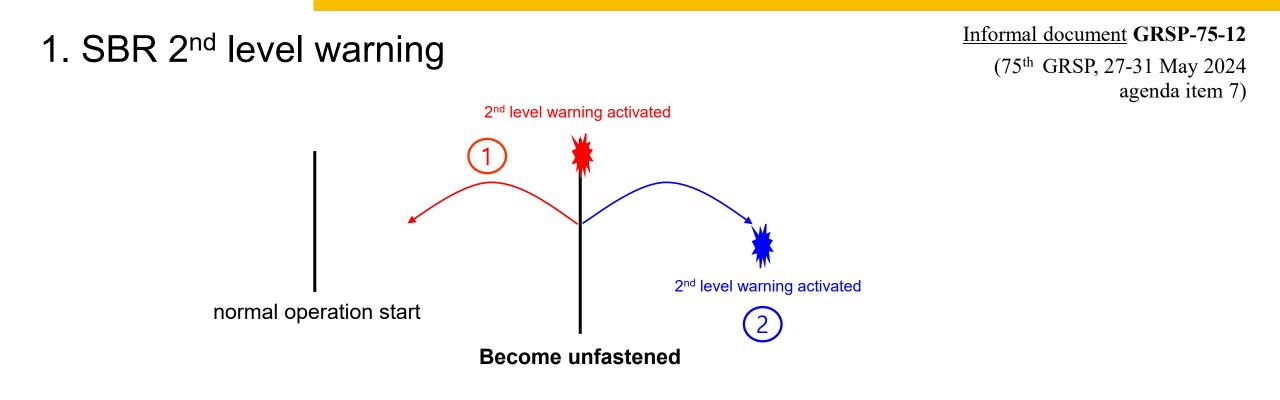
8.4.3.3. The second level warning shall be activated when a safety-belt is or becomes unfastened while the vehicle is in normal operation and while, at the same time, any one condition or any combination of the conditions, at the choice of the manufacturer, set out in paragraphs 8.4.2.4.1.1. to 8.4.2.4.1.3. is satisfied. >(1)
