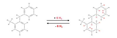
This means that, depending on the degree of hydrogenation, in one liter of benzyltoluene up to approximately 700 liters of hydrogen can be chemically bound.
