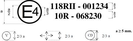
The above approval mark affixed to a component shows that the type concerned was approved in the Netherlands (E4) pursuant to Part II of UN Regulation No. 118 under approval number 001234 and Regulation No. 10<sup>1</sup> under approval number 068230.
