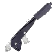
mechanical energy transmission to the parking brake e.g: handbrake lever
