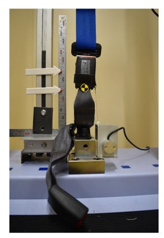
4. Perform a tensile test and measure the load and the movement of the buckle.
