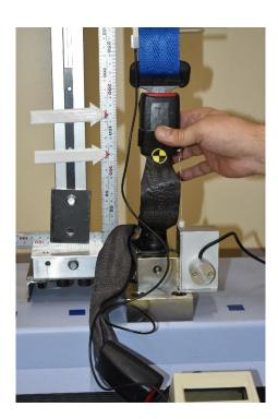
3. Attach the tongue to the buckle and set the belt of the tongue to the upper part of the tensile testing machine. The tension on the belt of the tongue is  $4 \pm 3$  N. After that, the buckle is released.
