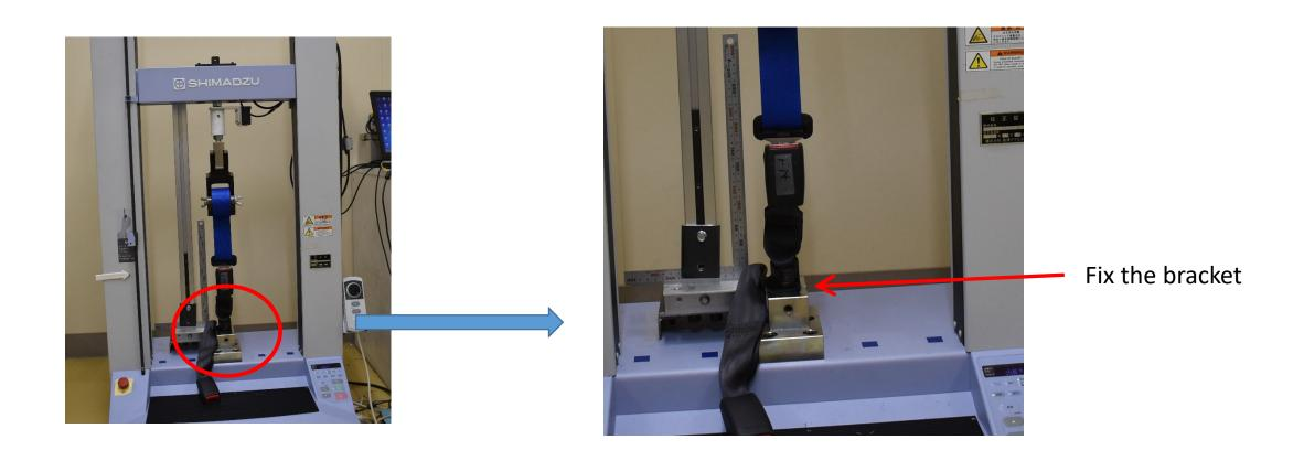
2. Fix the buckle at a position on the loading line of the tensile testing machine, that the distance between the buckle point and EA point is the same as the straight line distance between the EA and Bd point.
