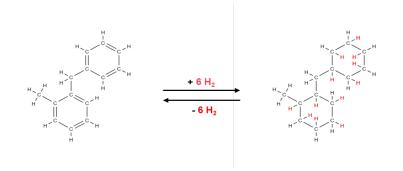
4. Special reaction conditions are necessary to later release the chemically bound hydrogen. In this specific case, the chemical bonds are released with the help of a catalytic system at temperatures of 250 °C. This means that the chemically bound hydrogen cannot be released under transport conditions.
