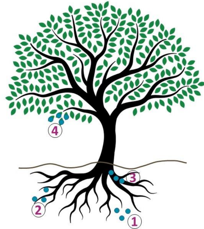
Figure: Phytoremediation of contaminated soil through 1) precipitation 2) root adsorption 3) root uptake 4) translocation
