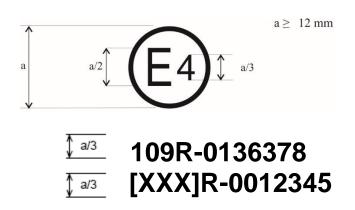
The above approval mark, affixed to a retreaded tyre according to paragraph 5.5. of this Regulation, shows that the concerned retreaded tyre is produced in a retreading production unit which has been approved in the Netherlands (E4) pursuant to UN Regulation No. 109 and that its type has been also approved in the Netherlands (E4) pursuant to UN Regulation No. [XXX]. The first two digits (01) of the approval number pursuant to UN
