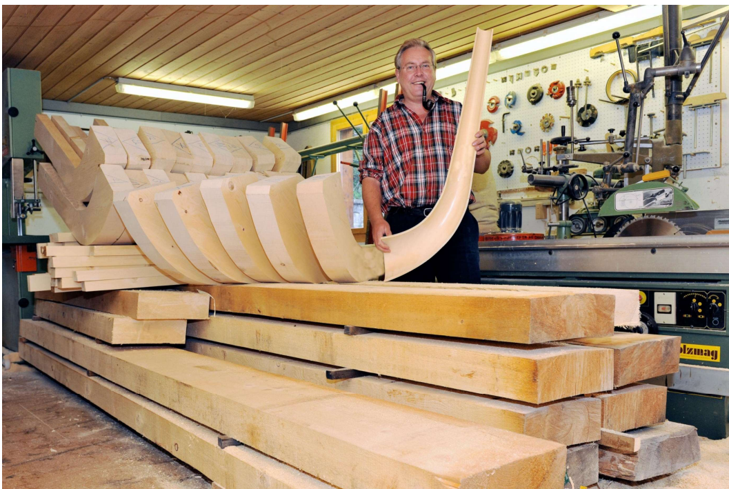
Fig. 33 Air-dried sheets of spruce moon wood, sawn workpieces and the finished tube end of an Alpine horn. (Image source: © Prix Lignum – photo by Beat Kollegger)
