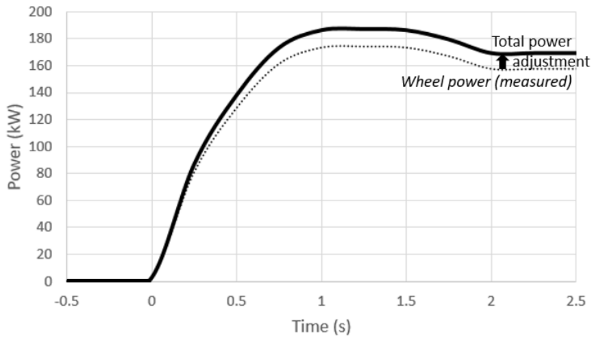
Figure 5 TP2 as measured wheel power adjusted for losses in gearbox
