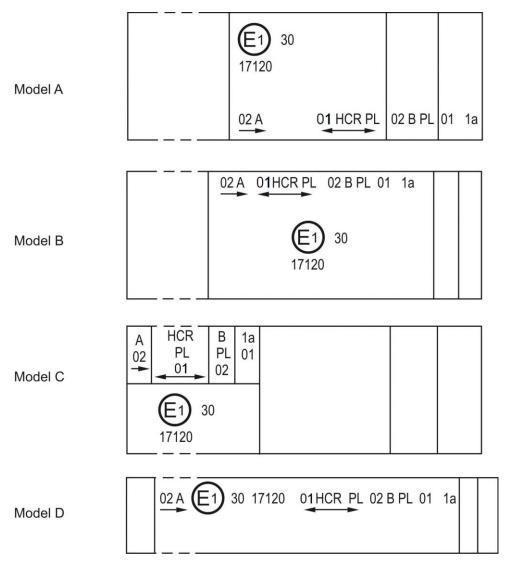
*Note:* The four examples above correspond to a lighting device bearing an approval mark comprising:
