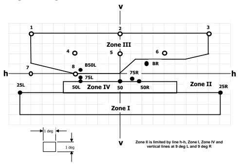
$h-h=horizontal\ plane$ ,  $v-v=vertical\ plane$  passing through the optical axis of the headlamp. The test point locations for left-hand traffic are mirrored about the VV line.
