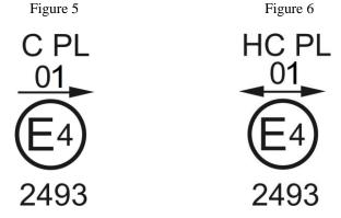
The headlamp bearing the above approval mark is a headlamp incorporating a lens of plastic material meeting the requirements of this Regulation in respect of the passing-beam only and is designed:
