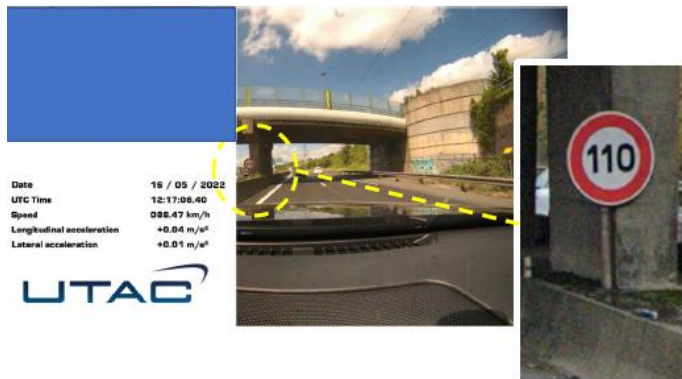
Traffic sign mis use– adjacent lane
