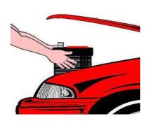
After the Change of the 12V Battery, the Battery-Management-System must be activated.
