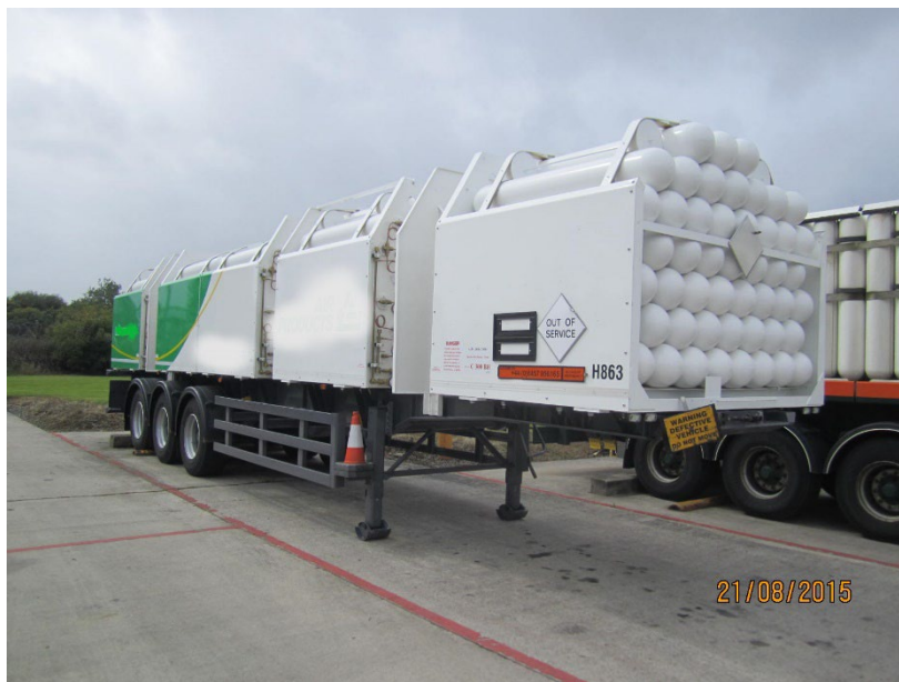
Battery-vehicle constructed with seamless steel cylinders
