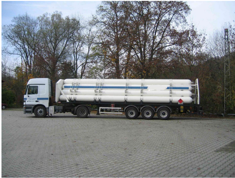
Battery-vehicle constructed with seamless steel tubes
