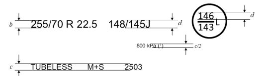
(1) PSI marking instead of kPa is allowed for tyres first type approved before 1 January 2018. The kPa marking may be preceded by "TEST AT:" or, alternatively, by "TEST INFL:" or the symbol "@".
