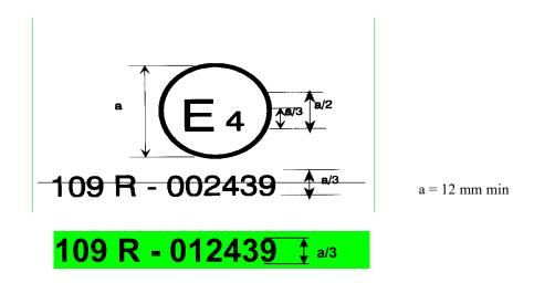
The above approval mark affixed to a retreaded tyre shows that the retreading production unit concerned has been approved in the Netherlands (E4) under approval number 109R0012439 meeting the requirements of 01 series of amendments to this Regulation in its original form (00).
