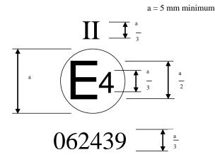
The above approval mark affixed to a device for indirect vision indicates that the device is a main rear-view device, of Class II, which has been approved in the Netherlands (E 4) pursuant to Regulation No. 46 and under approval number 062439. The first two digits of the approval number indicate that Regulation No. 46 already included the 06 series of amendments when the approval was granted.
