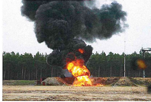
Test set-up for external fire test, full fire phase (maximum flame) after ignition.
