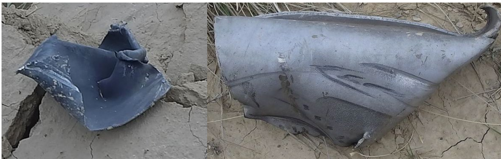
Figure 4: Fragments of the tank after the test.
