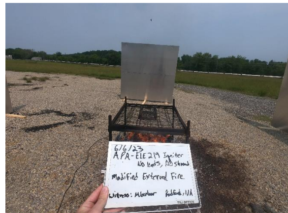
Figure 19. External Fire Test, post-test
