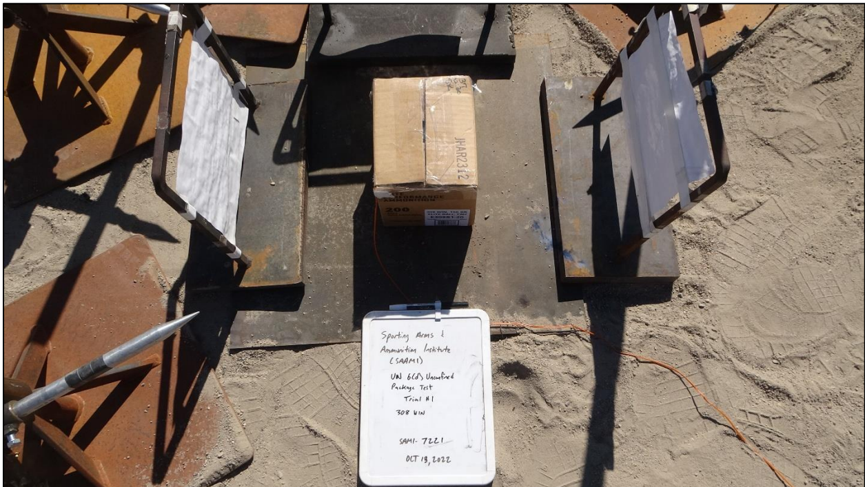
Photo 15: Representative Unconfined Package Test Setup – Sig Sauer 308 Win
