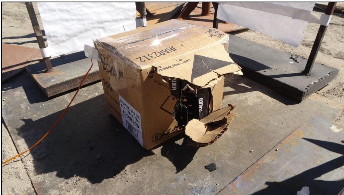
Photo 24: Unconfined Package Test Results – Sig Sauer .308 – Trial 1
