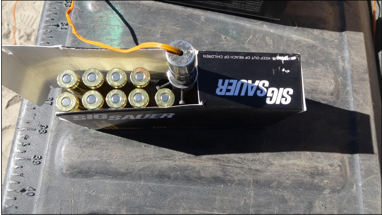
Photo 14: Intermediate Package Prepared with Igniter – Sig Sauer 308 Win
