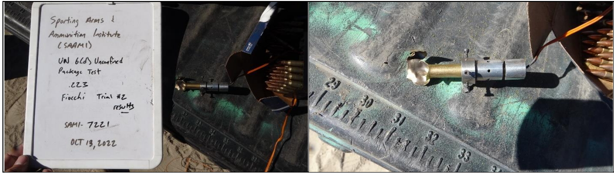
Photo 20: Unconfined Package Test Results – FIOCCHI .223 – Trial 2
