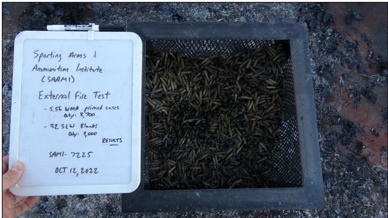
Photo 22: UN Series 6 (c) External Fire Test #2 Results
