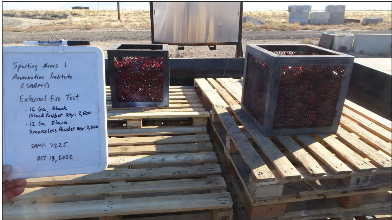
Photo 16: UN Series 6 (c) External Fire Test #3 Setup
