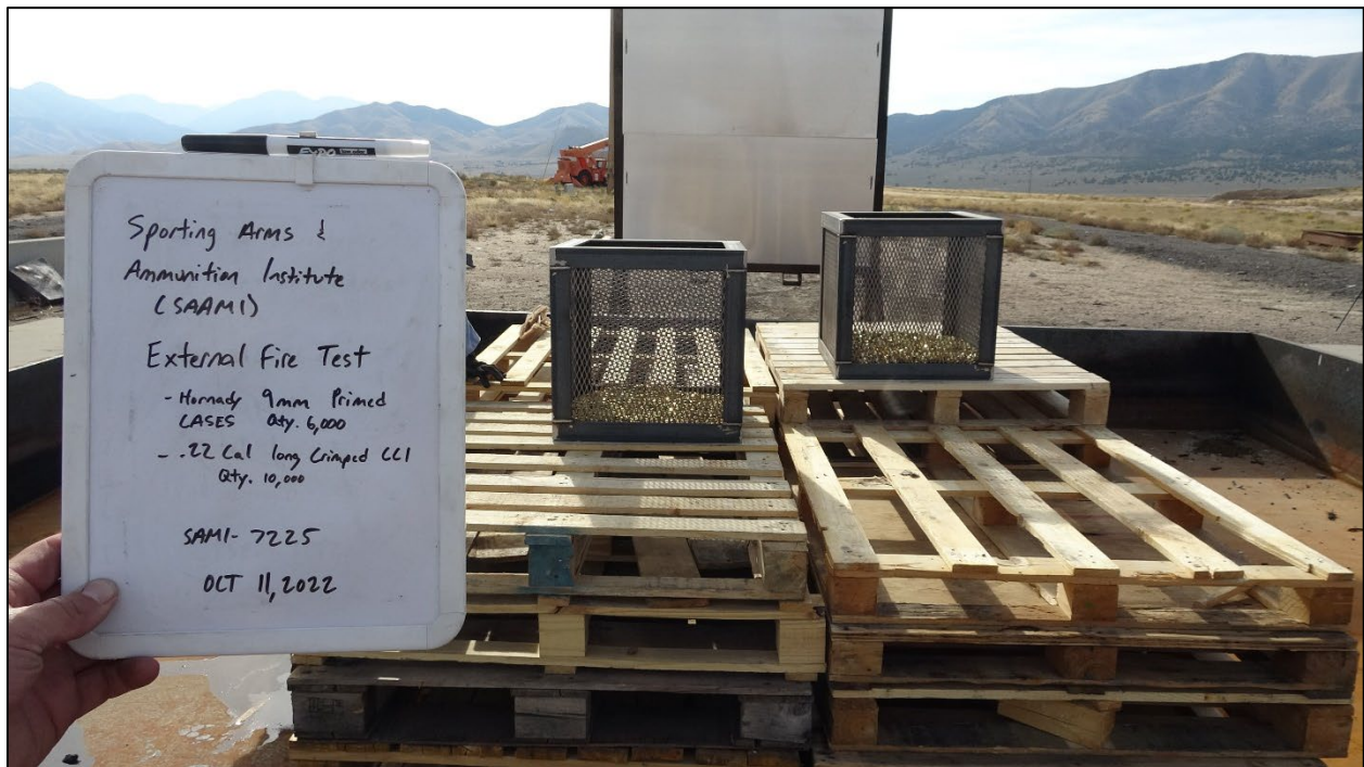
Photo 14: UN Series 6 (c) External Fire Test #1 Setup
