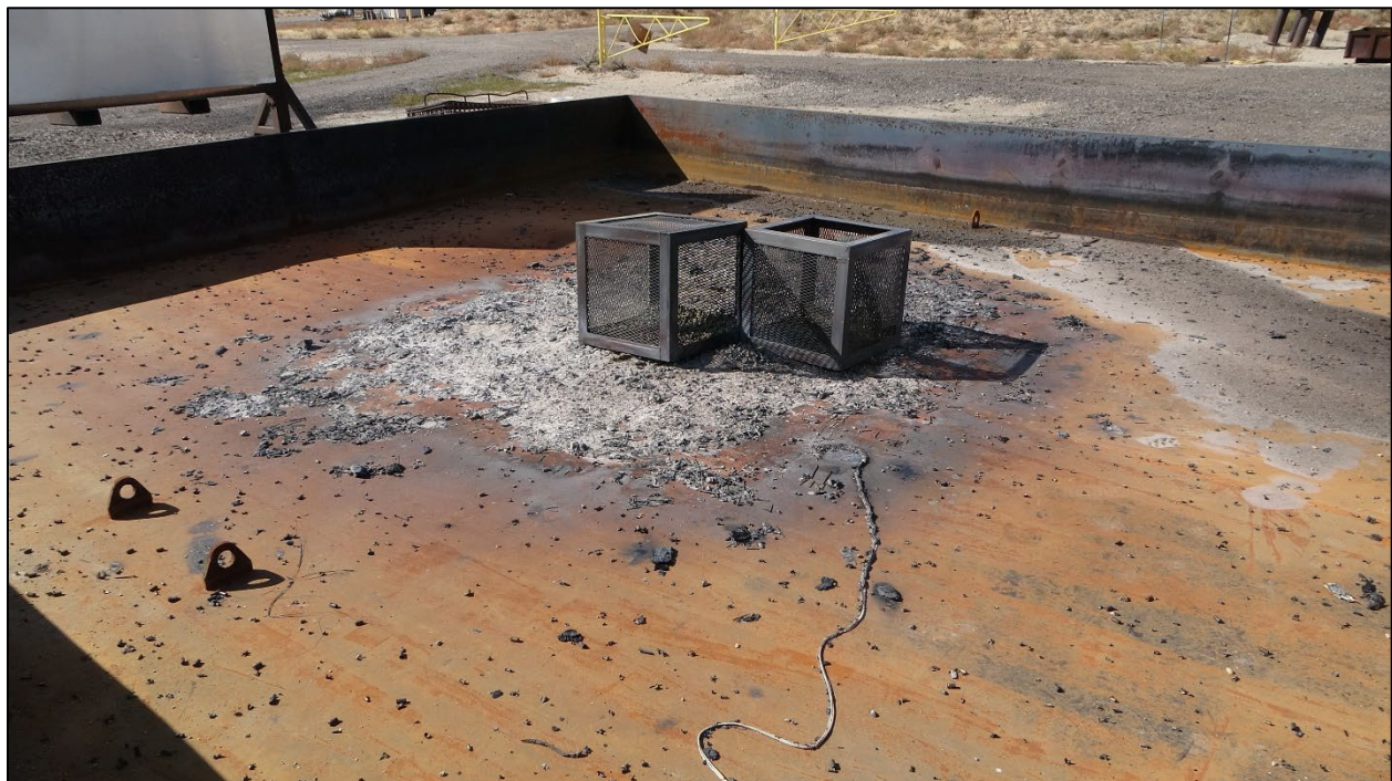
Photo 18: UN Series 6 (c) External Fire Test #1 Results
