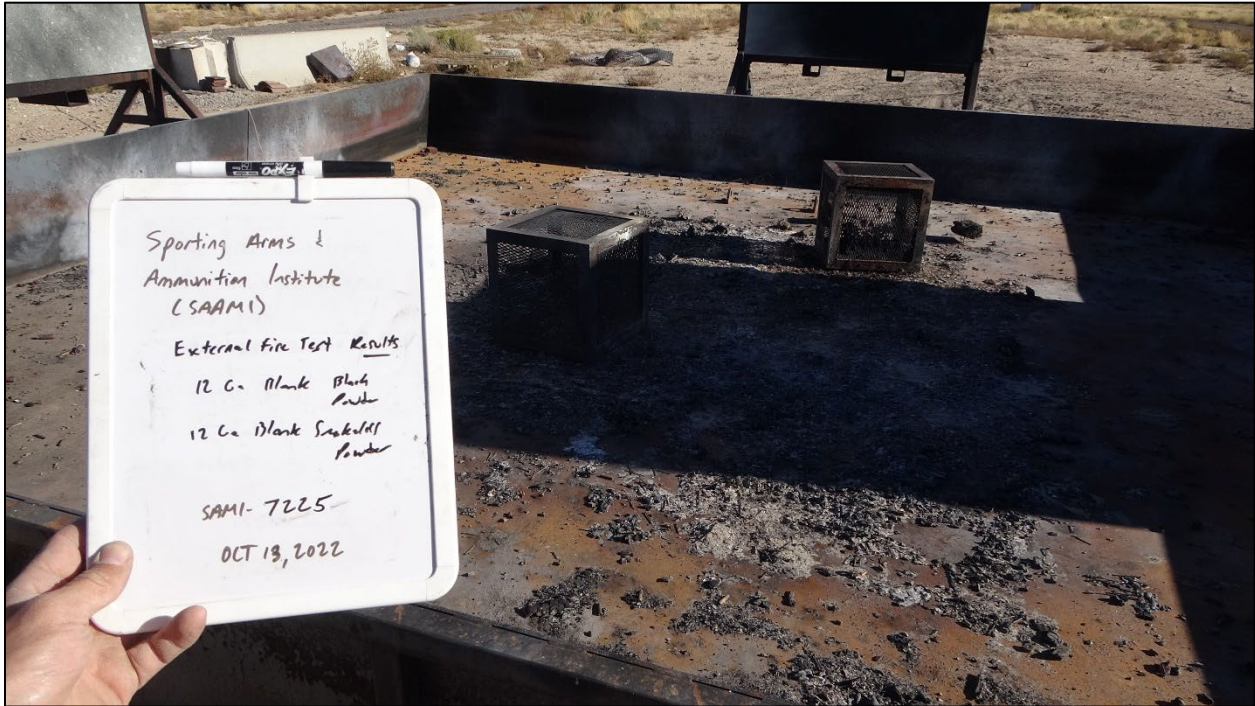
Photo 23: UN Series 6 (c) External Fire Test #3 Results
