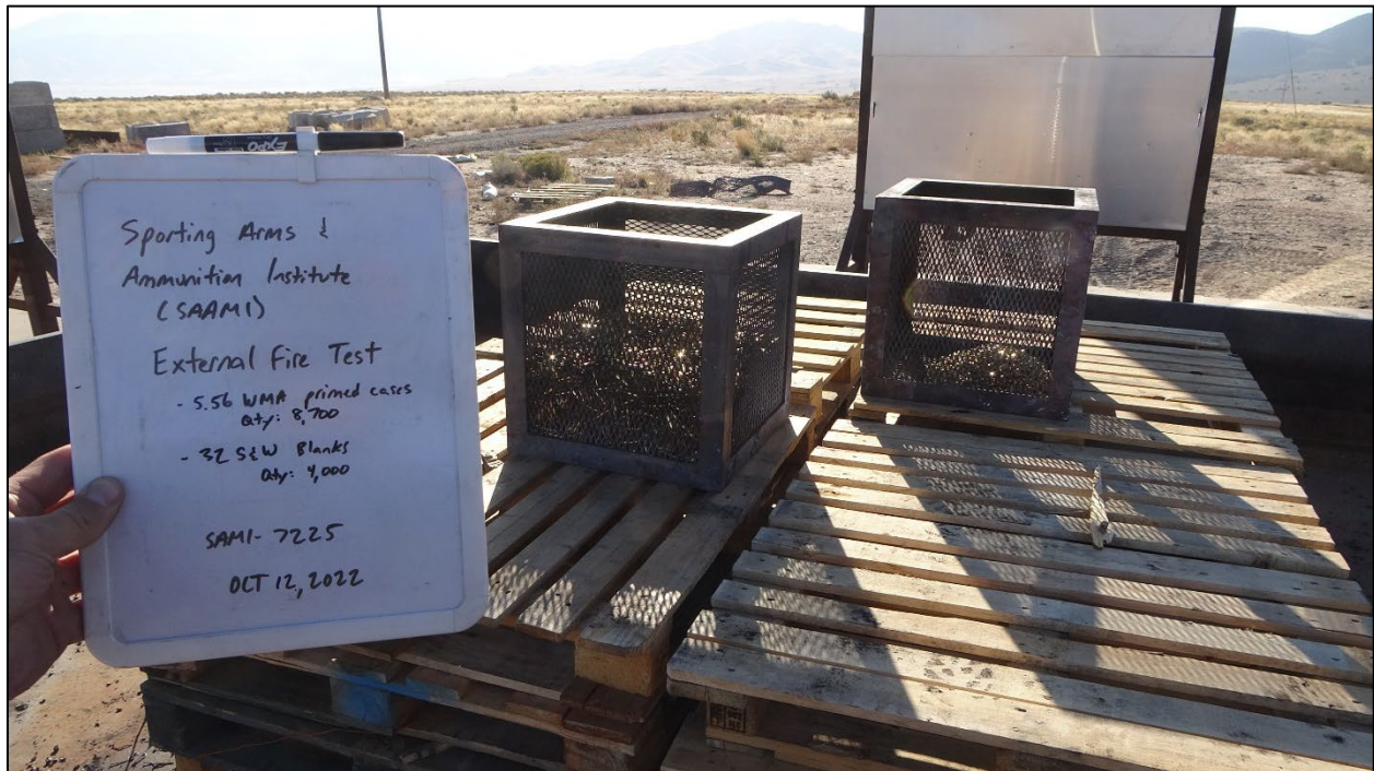
Photo 15: UN Series 6 (c) External Fire Test #2 Setup
