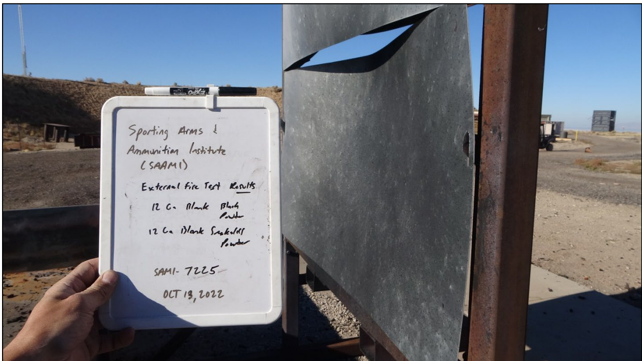
Photo 24: UN Series 6 (c) External Fire Test #3 Results
