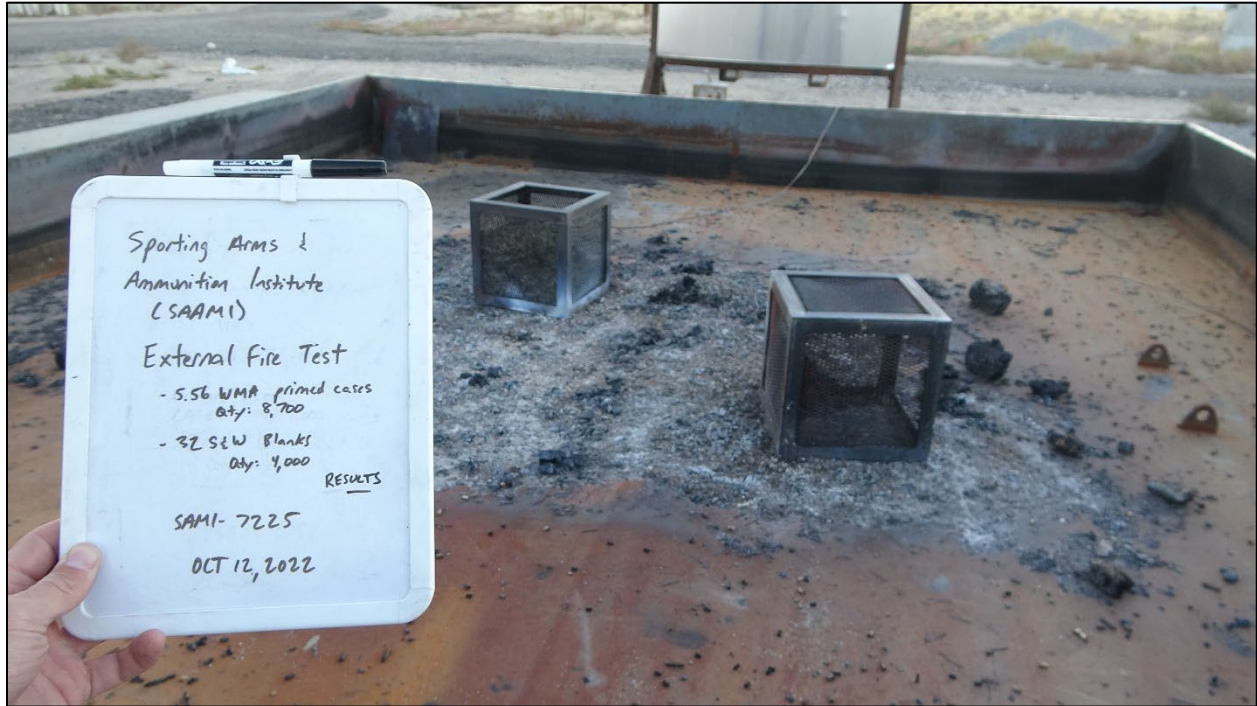
Photo 21: UN Series 6 (c) External Fire Test #2 Results
