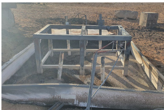
Figure 5: Modified tanker stand after test
