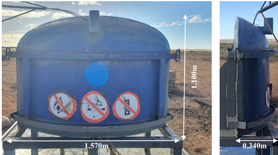
Figure 2: Pup tanker trailer after modification
