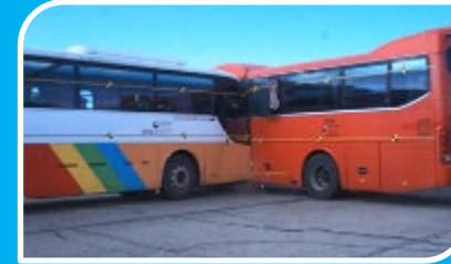
[30km/h HDV-HDV side crash test]
