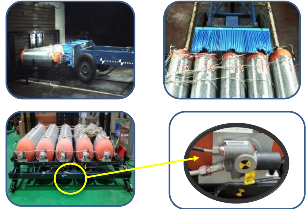
<40km/h CHSS module (w/o P) impact test in longitudinal direction (LTD)>
