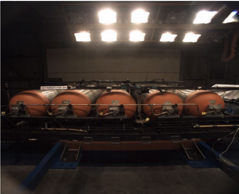
<Sled test based on crash acceleration>
