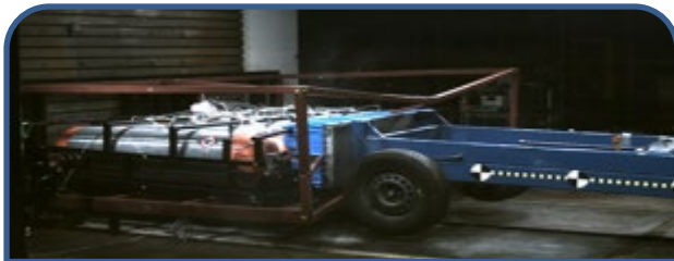
<CHSS module test with protective structure>
