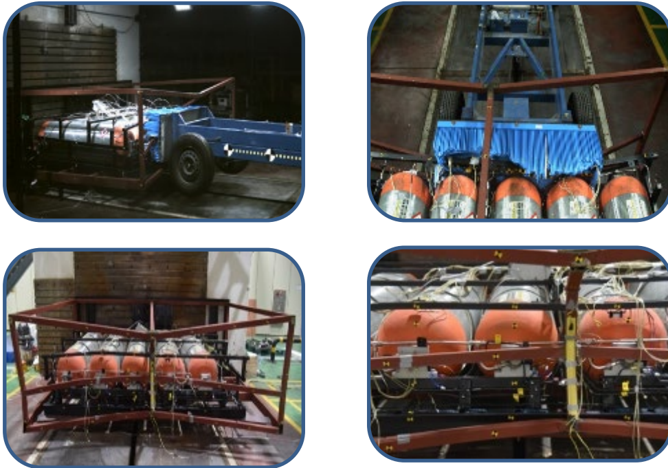
<50km/h CHSS module impact test (w/ P) in longitudinal direction (LTD)>
