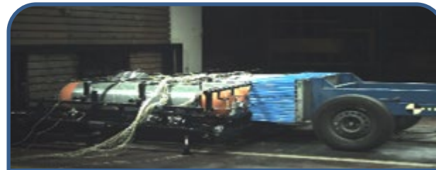
<CHSS module test in longitudinal direction >
