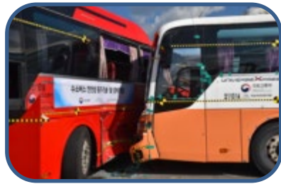
<30km/h HDV-HDV side crash test>
