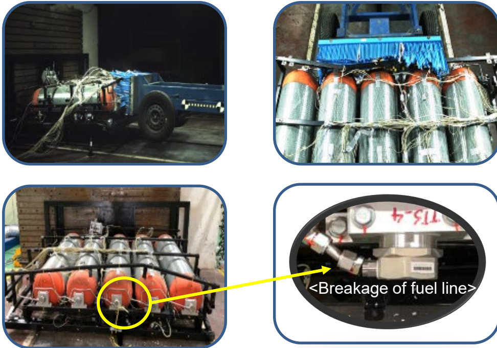
<50km/h CHSS module impact test (w/o P) in longitudinal direction (LTD)>
