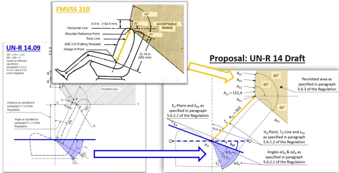
For the permitted area during and after the test, a new area must be defined for the upper belt anchorages as otherwise the current provisions regarding the CY-line can very likely not be fulfilled. The idea is to create a permitted area, whose lower boundary is limited to a distance of min. 450 mm around the  $H_R$  point.
