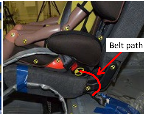
Figure 2 Photo of the Buckle Strap Path When Not Straight
