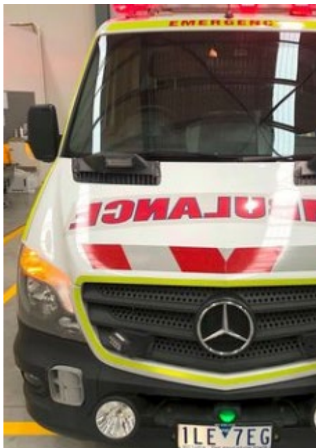
Figure 5: Green operational lamps to help traffic cameras recognise when emergency service vehicles have activated their flashing lights to respond to an emergency. The green light remains on because there's a chance the traffic cameras will miss the rapidly flashing blue and red lights as they pass.
