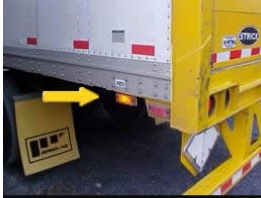
Figure 2: Operating status lamp for ABS on a trailer
