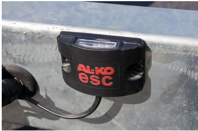
Figure 3: Operating status lamp for Electronic Stability Control (ESC) on a trailer
