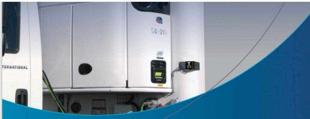
Figure 4: Operating status lamp for a cooling system on a refrigerated trailer
