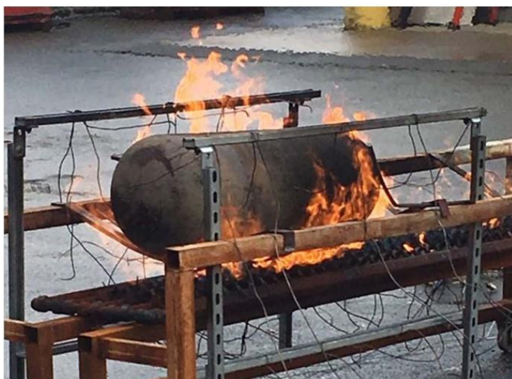
Figure 13 Containers in a Fire Testing
