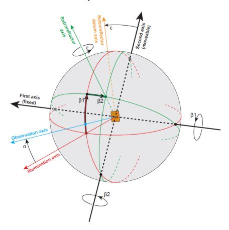
3.2. An adequate support (goniometer) is demonstrated in Figure A4-II. It represents a goniometer mechanism embodying the CIE angular system for specifying and measuring retro-reflective device and marking materials. All axes, angles, and directions of rotation are shown positive.
