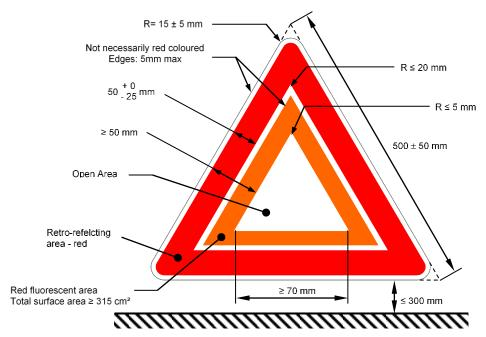
$\label{thm:continuous} Figure~A5-IX\\ \textbf{Shape and dimensions of the advance warning triangle of type 2 and of the support}$
