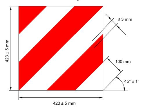
Figure A5-IV **Retro-reflective material marking of Class 5**
