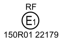
$\label{eq:Figure A10-V} \textbf{Arrangement of the approval mark for advance warning triangle}$
