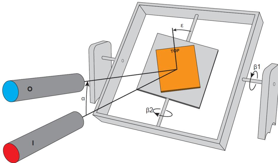
3.3. For testing the retro-reflection the retro-reflective devices shall be illuminated with a CIE Standard Illuminant A (ISO 11664-2:2007(E)/CIE S 014-2/E:2006) and measured as described in Part 1 of Annex 4.
