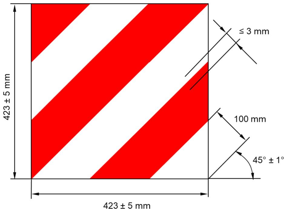
6. Shape and dimensions of HLV retro-reflective marking plates of Class 1, 2, 3 or 4
