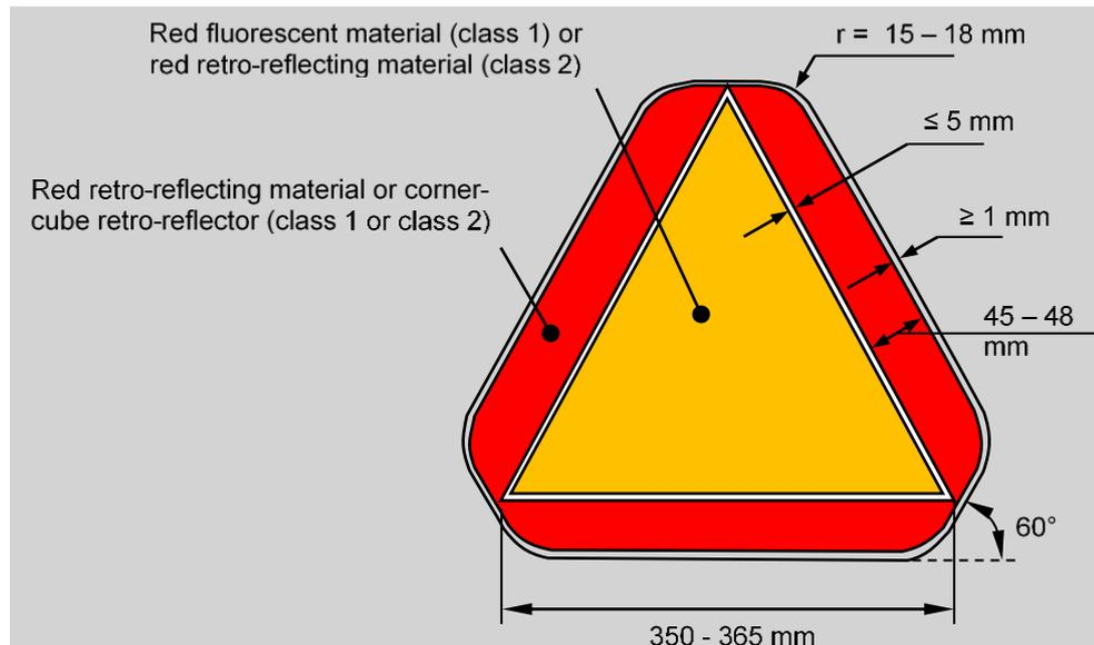
8. Shape and dimensions of the advance warning triangle Type 1 or 2 (Figure A5-VIII or A5-IX)
