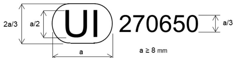
The above Unique Identifier marked on the retro-reflective device shows that the type concerned has been approved and that the relevant information on that type approval can be accessed on the UN secure internet database by using 270650 as the Unique Identifier.
