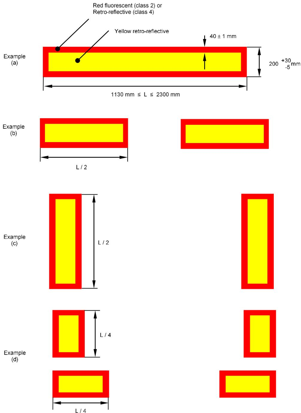
7. Shape and dimensions of SMV retro-reflective marking plates of Class 1 or 2
