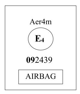
The ... 06, 07, or 08 or 09 series of amendments at the time of the approval. This safety-belt has to be fitted to a vehicle equipped with an airbag in the given seating position."
