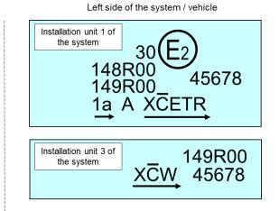
The system bearing the above approval markings meets the requirements of this Regulation (original version of the Regulation) in respect of both a passing-beam for left-hand traffic and a driving-beam with a maximum intensity comprised between 123,625 and 145,125 candelas (as indicated by the number 30) grouped with a front direction indicator lamp of category 1a and a front position lamp approved in accordance with the 00 series of amendments of UN Regulation No. 148.
