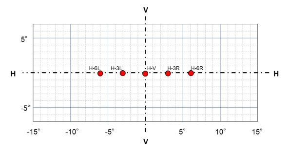
Figure A4-IV Secondary driving-beam Class CS and DS - position of test points
