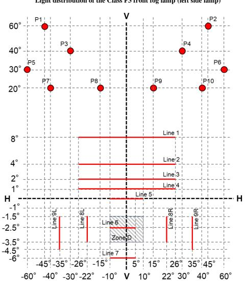
Figure A4-X Light distribution of the Class F3 front fog lamp (left side lamp)
