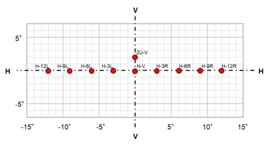
Figure A4-III Driving-beam Class BS - position of test points
