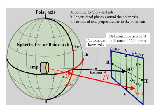
Figure A4-I Spherical coordinate measuring system
