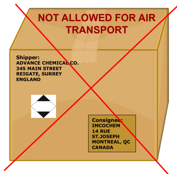
Figure 3.4.2: Limited quantity for transport modes other than air (not acceptable for air) in accordance with paragraph 3.4.7 of the Model Regulations
