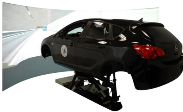
Figure 5 AS1200-6 passenger car simulator.
