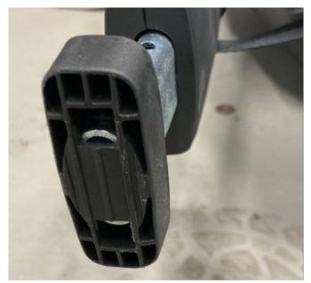
Foot dimensions fulfil requirements of paragraph 6.3.5.3. but effectively, only the <u>footprint of the tube</u> spreads the loads accross the vehicle structure creating a "pinpoint load"
