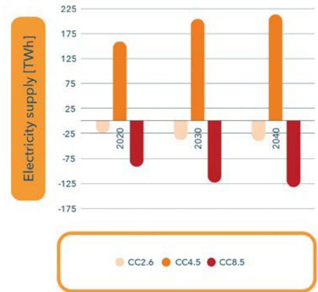
Figure 7. Climate Change impact on power supply from cascade HPPs in the HPPDev scenario, under different RCPs.
