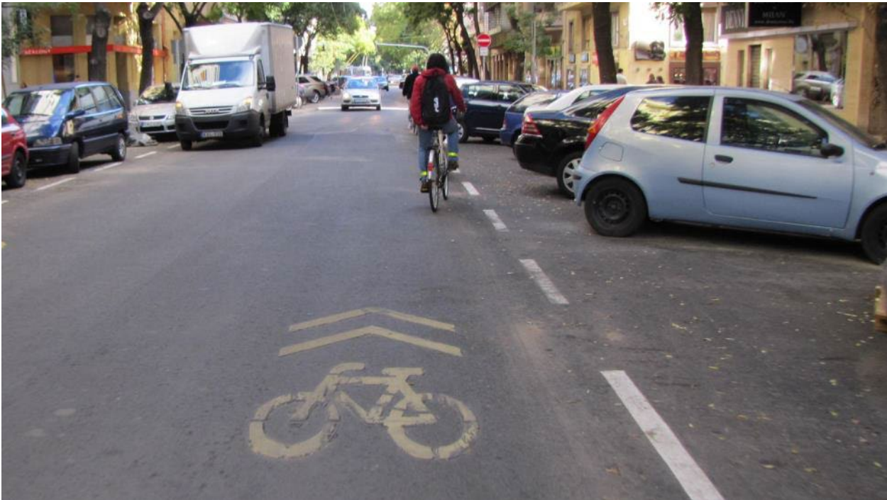
Figure 4. Example use of sharrows in a street with contraflow cycling. Budapest, Hungary. Source: Aleksander Buczyński
