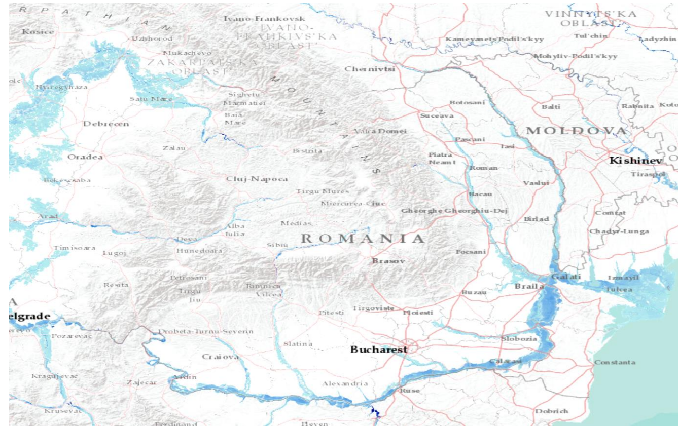
Figure 4. Flood hazard map of Romania - Return period of 500 years (Dottori et. al, 2016)
