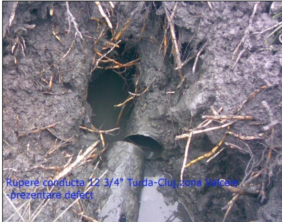
Figure 13. Gas pipelines affected by landslides – area 2
