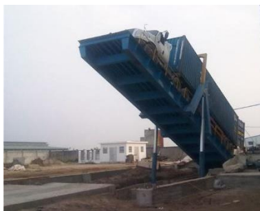
Figure 7.87 Plateau basculant 100 t
