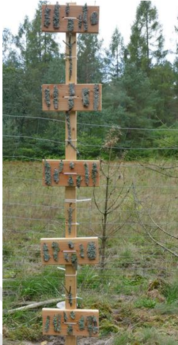
Figure 18: Exposure boards with Hypogymnia physodes in heights between 0.2 m and 2 m in Sandkrug
